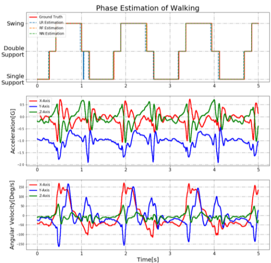
Fig. 2: Performance of three models on walking task. (Top) The ground truth and estimation of three models. (Middle) 3-axis acceleration during walking. (Bottom) 3-axis angular velocity during walking. LR model sometimes produces erroneous estimation while RF and NN perform very well.
